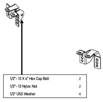
Place the provided space mount into the frame end as shown. Use the provided spacers on the outside edges when mounting the winch mount in the next step.
