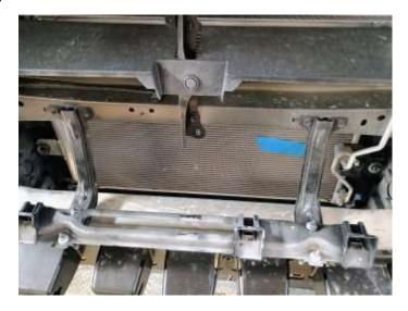
Undo the clips hold the bumper to the shroud as shown. Remove the bumper by unbolting the assembly at the frame and bumper side wings (located behind the arrow below). Save hardware for reuse.
