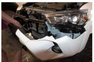
Remove the lower front cover by undoing the clips holding it in place
