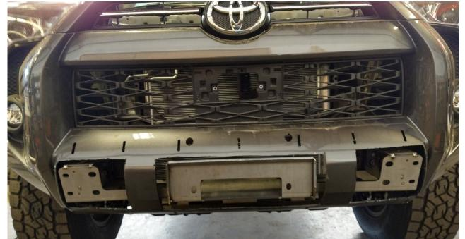
Cut out openings once template is traced. Reinstall once mounting brackets and internal are mounted.
