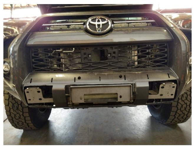
Use the provided 3/8" clip nuts to attach the cover to the vehicle and internal mount using the provided 3/8" hex cap bolts. Leave hardware loose for adjustment and alignment of the mounts before tightening.
