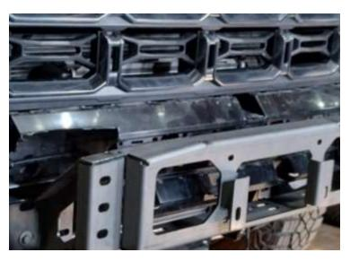
The plastic below the grille may need to be trimmed in some cases to allow the winch and its external parts to clear. DO NOT cut off completely as the tab openings on the edge of the grille will remount your OEM fascia piece
