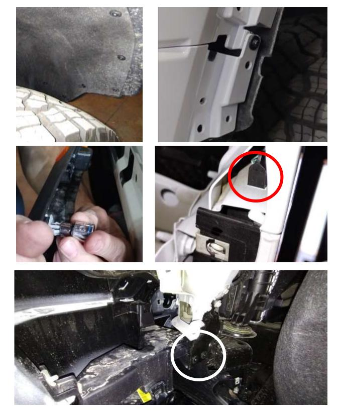
Unbolt the rear of plastic fascia, also detach the grille by removing the plastic shroud and hardware. Undo all wiring and check for connections before removing the bumper.
