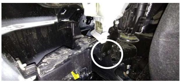
Unbolt the rear of plastic fascia, also detach the grille by removing the plastic shroud and hardware. Undo all wiring and check for connections before removing the bumper.
