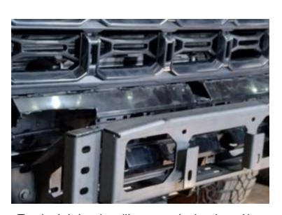
The plastic below the grille may need to be trimmed in some cases to allow the winch and its external parts to clear. DO NOT cut off completely as the tab openings on the edge of the grille will remount your OEM fascia piece
