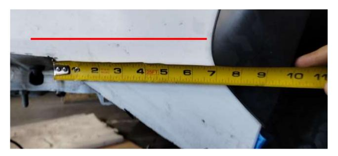
Continue cutting until 10" from the wheel opening and about an 1" down from the bumper transition line. The diagonal cut line will meet up with the cuts shown below. Measure 2" down from the edge of the wheel well trim and over  $2 \frac{1}{2}$ ". At this time drill a few  $\frac{1}{4}$ " holes for a bracket to be installed later (not dependent on preciseness). Reattach bumper after brackets are installed.
