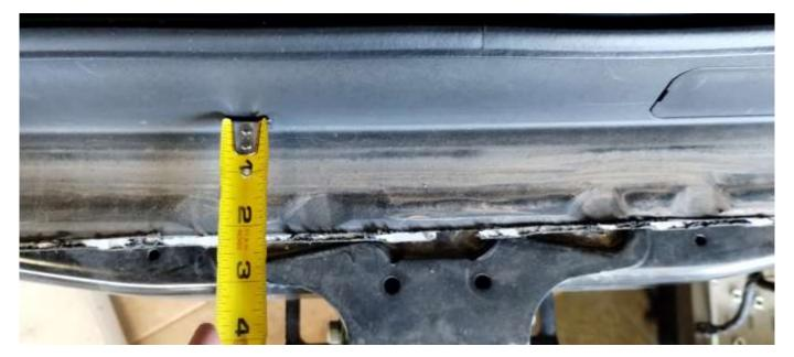
Cut both the OEM bumper and plastic tread piece (recommend separating) about 2 1/4" from the load floor As shown. Tread plate on new bumper will slide over this region
