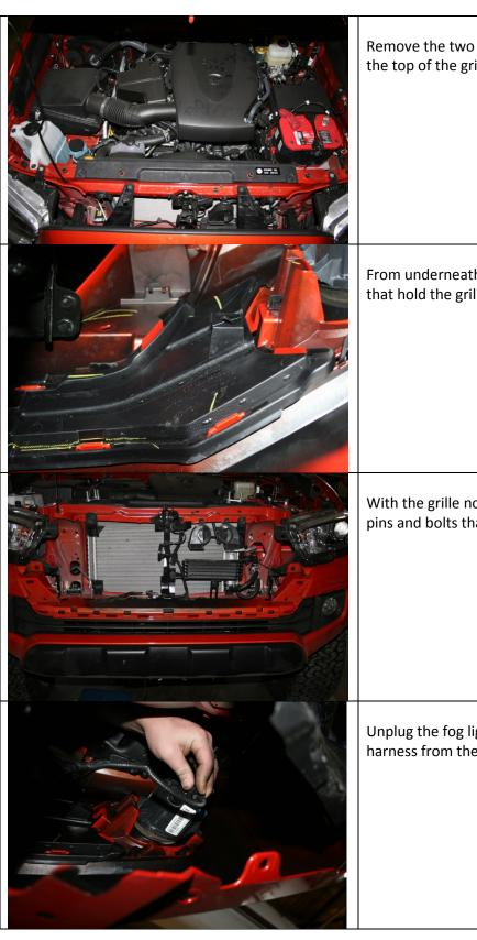
Remove the two bolts and two clips that retain the top of the grille.
