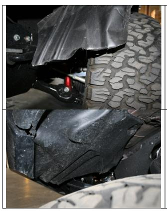
Trim the bottom of the inner fender well off as shown.
