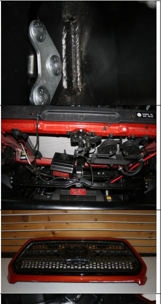
Lift the bumper into place and install the three bolt plate into the mounting hole with the studs face the center of the vehicle this will allow for easy tightening of the bolts.
